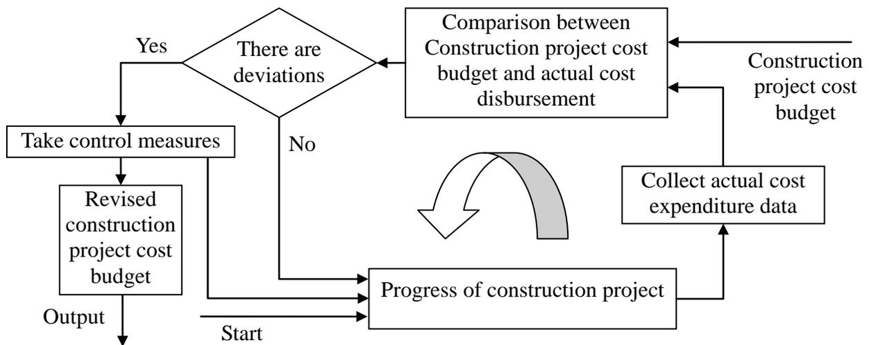
Fig. 1. Process on construction project cost control
